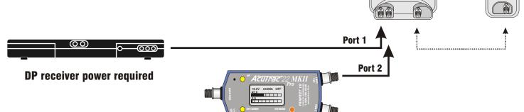
Use of the internal battery for powering the DishPro Plus LNBF will drain the battery very rapidly and may ultimately result in a short life span for the battery and/or premature failure of the meter itself; therefore it is not recommended.
