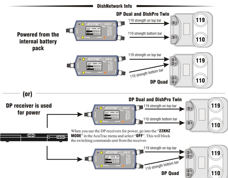
The DP receiver sends out a "switch" command whenever it is not locked on a satellite, obviously, this is the case if the antenna is not aligned yet. This command causes the dual or quad LNBF to switch from one output (say 110) to the other (say 119). When aligning the antenna, this can be pretty confusing so block the switch command in the AcuTrac22Pro MKII by turning the 22KHZ "OFF" when a dual or quad LNBF is attached and a DP receiver is used for power.
