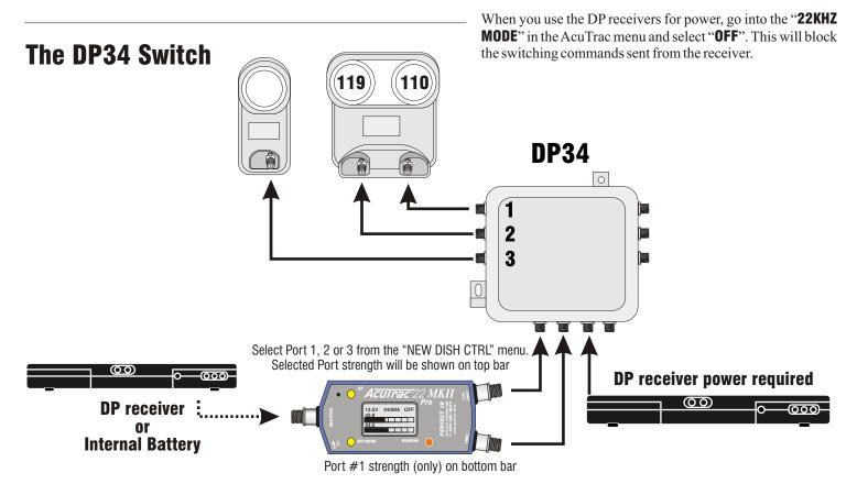
The DP34 and its components draw a considerable amount of current, typically in excess of 600 mA. Since this approaches the upper current limit of the AcuTrac22Pro MKII, it is recommended that you use a DP receiver to power hardware. (make this connection first). This will reduce the mA draw on the AcuTrac22Pro MKII considerably. A second receiver may optionally be used to power the AcuTrac if the internal battery level is low in the meter.
