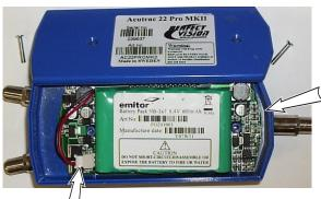
Disconnect old battery Connect new battery Replace bottom cover
