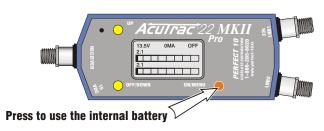
strength indicated on the bar graph(s) by minor azimuth, elevation and skew adjustments of the dish. When you have maximized the readings, lock the dish mount bolts and re-attach the LNBFs to the switches or cables provided with the antenna. Then check your efforts with the satellite receiver.
