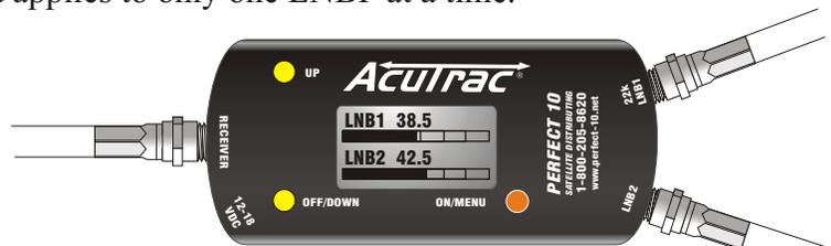
Press the “**OFF/DOWN**” button once. The tone will begin and the letter ‘T’ will appear above the top bar graph. This indicates that the tone applies to the top LNB reading.
