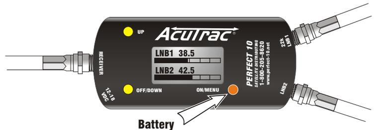
The signal strength is indicated in digits just above each bar graph. As you move the dish, you will see the increase and decrease in signal strength. The objective is to maximize the signal reading on both bar graphs by minor azimuth, elevation and rotation adjustments. When you have maximized the readings, lock the mount bolts. Re-attach the LNBs to the switches or cables provided with the antenna. Then check your efforts with the satellite receiver.
