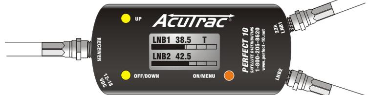
To apply the tone to the bottom LNB, press the “**OFF/DOWN**” button once more. The ‘T’ will appear above the bottom bar graph and the tone will apply to that LNB. To cancel the tone, press the “**OFF/DOWN**” button one more time.
