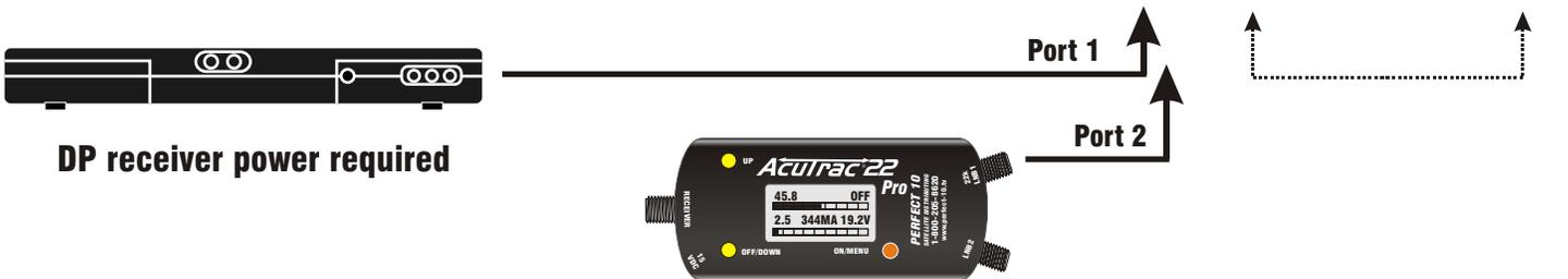
Use of the internal battery for powering the DishPro Plus LNBF will drain the battery very rapidly and may ultimately result in a short life span for the battery and/or premature failure of the meter itself; therefore it is not recommended.
