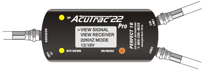
**VIEW SIGNAL** This is the screen you will see when you first turn the AcuTrac22 Pro on. These bars indicate the general signal strength, voltage and current draw in mA of all connected devices. If desired, you can look at only one LNB by pressing the “**UP**” button. Press the “**UP**” button again to look at only the second LNB, one more press of the “**UP**” button takes you back to both LNBS.
