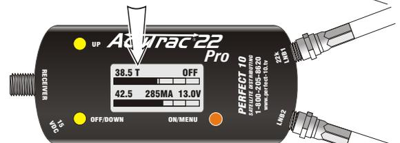
To apply the tone to the bottom LNB(2), press the **“OFF/DOWN”** button once more. The 'T' will appear above the bottom bar graph and the tone will apply to that LNB. To cancel the tone, press the **“OFF/DOWN”** button one more time.
