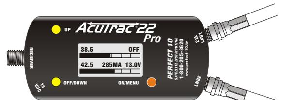
Press the **“OFF/DOWN”** button once. The tone will begin and the letter 'T' will appear above the top bar graph. This indicates that the tone applies to the top LNB(1) reading.
